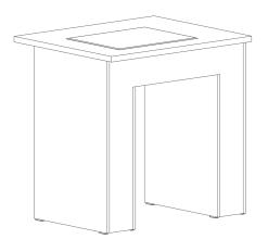
The function of weighing tables in both ST and LM versions is identical. The difference lies in the material used to fill the structure. The ST version uses sheet steel panels, customized according to the type and colour of the casework in a particular laboratory. The LM version is finished with laminated particle board. The tables can be additionally equipped with a practical drawer.
